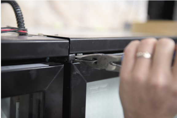
FIGURE 28: Use a Wedge & Pinch Hinge Pin
