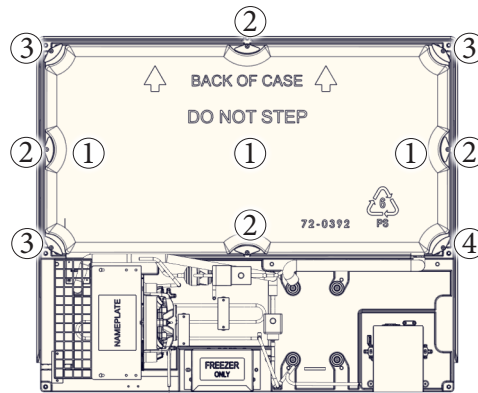
FIGURE 50: Evaporator Cover Bolt Torque Pattern
