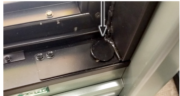
FIGURE 36: Torque Adjuster Plug
