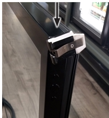
FIGURE 26: Remove Hinge Pin
