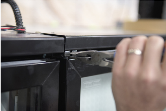
FIGURE 24: Use a Wedge & Pinch Hinge Pin
