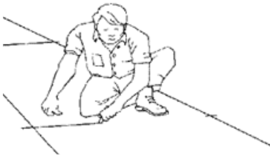
FIGURE 5: Measure and Mark Exact Case Outline
