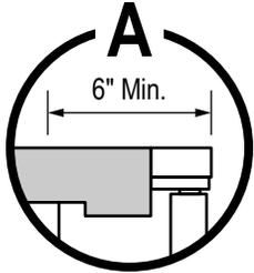
Building soffits must be set back at least 6" from the front of the doors to allow access to electrical wiring on the top of the case.
