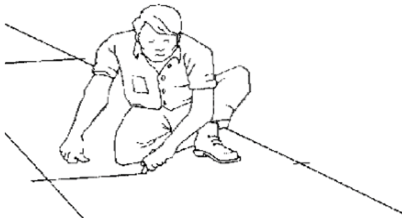
FIGURE 4: Measure and Mark Exact Case Outline
